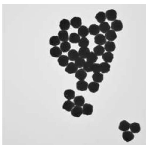
IMAGE - Transmission Electron Microscopy of the Colloidal Gold Nanoparticles. Colloidal Gold Nanoparticles Were Manufactured As Described In The Materials And Methods
