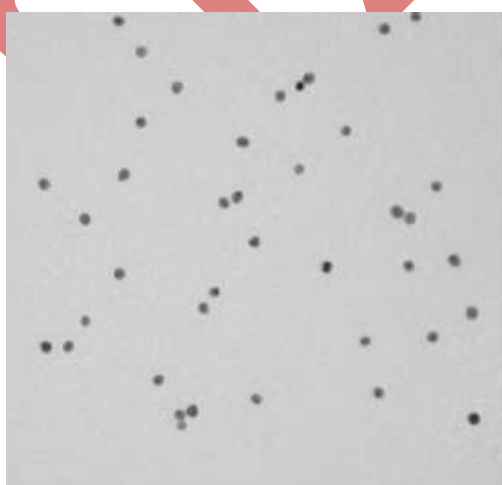
IMAGE - Transmission Electron Microscopy of the Colloidal Gold Nanoparticles. Colloidal Gold Nanoparticles Were Manufactured As Described In The Materials And Methods
