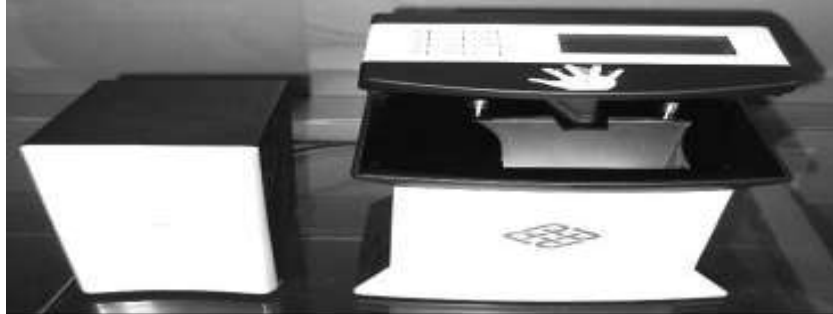
Figure 2: A CCD-based palm print scanner
