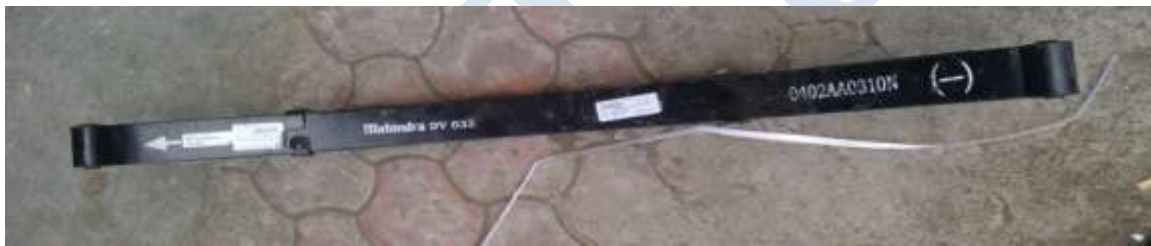
Figure No. 1 Mahindra Bolero Rear Leaf Spring
