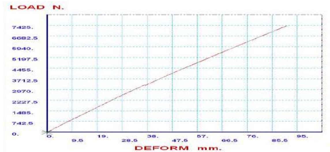
Graph No. 3 Testing mono composite leaf spring (load vs. deflection)
