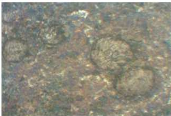
Figure 3 SG Iron specimens (at 860^{\circ}\text{C} Austempered)
