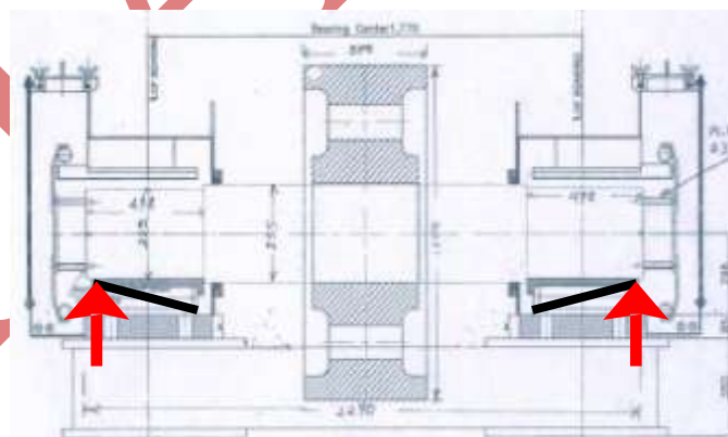
Case 3. Right and Left Bushing Nonparallel to the Shaft Journal
