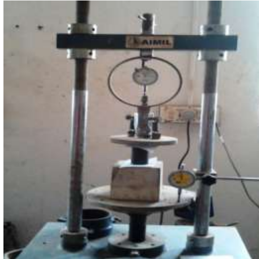
Fig.3 Laboratory UCS Test Set Up
