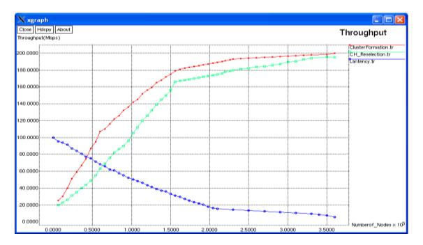
The end to end delay decreases when throughput of the cluster formation and cluster head reselection increasing in the network.
