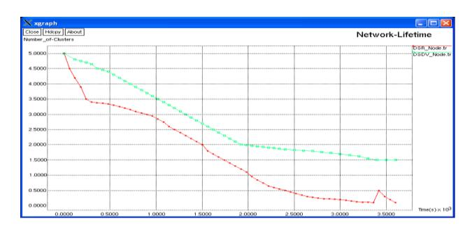
Using this graph, DSR protocol formation of cluster is less compare to the DSDV protocol based on time (s). So network lifetime easily judge to the best protocol.
