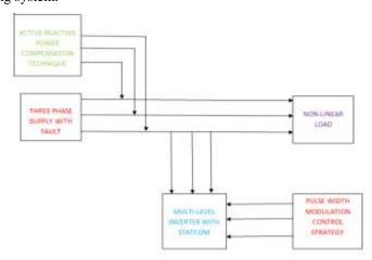
The STATCOM is utilized to identify the faults and compensate those faults in order improve the system performance. It is maintained and controlled with use of proper controlling pulses from the pulse width modulation control strategy. Here the usage of inductance and common dc –link capacitor are performed to
