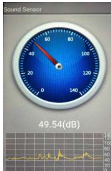
Fig.6: Sound sensor with its run lime graph measured in dB.
