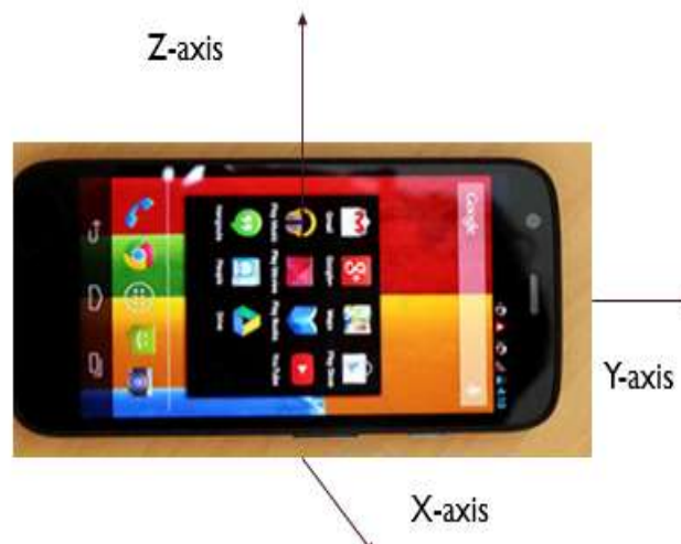
Fig.1: Moto G and Three-axis diagram of the accelerometer. It employs a LIS3DH 3-axis accelerometer, which is capable of detecting movement in any direction. This movement may be the slightest deviation or a disturbance caused by a external environment
