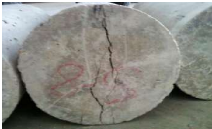
Fig.7 Specimen Failed in Tension (vertical crack is appeared)
