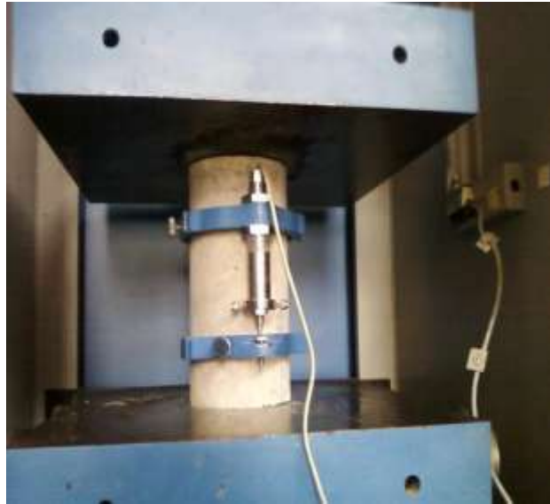
Fig.8 Set to Draw Stress Strain Curve by CTM Using LVD
