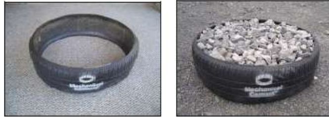
Fig.1. Tire Tread Cylinder used for CA concrete
