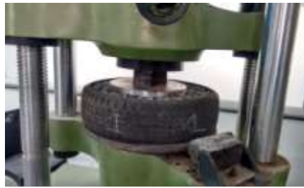
Fig.2. CA Concrete under Compressive Force
