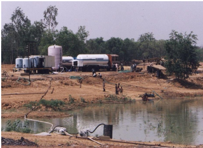
Figure 6: Liquid Nitrogen Flushing, Foaming Nitrogen Flushing and Portable PSA Nitrogen Generator at Jhanjra Project, West Bengal, India. (Photograph by Voráček)
