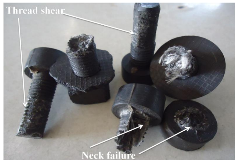
Figure 5. UPR-100/GFS-50/GFL50 composite fasteners (M14 x 2) size showing the fracture under the tensile load.
