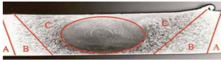
Fig. 2. Micro structural zone classification in a friction stir weld (A: parent material, unaffected by process; B: HAZ, thermally affected but with no visible plastic deformation; C: TMAZ, affected by heat and plastic deformation) .
