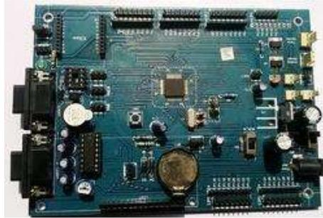
Fig 2: ARM LPC2148 microcontroller unit.
