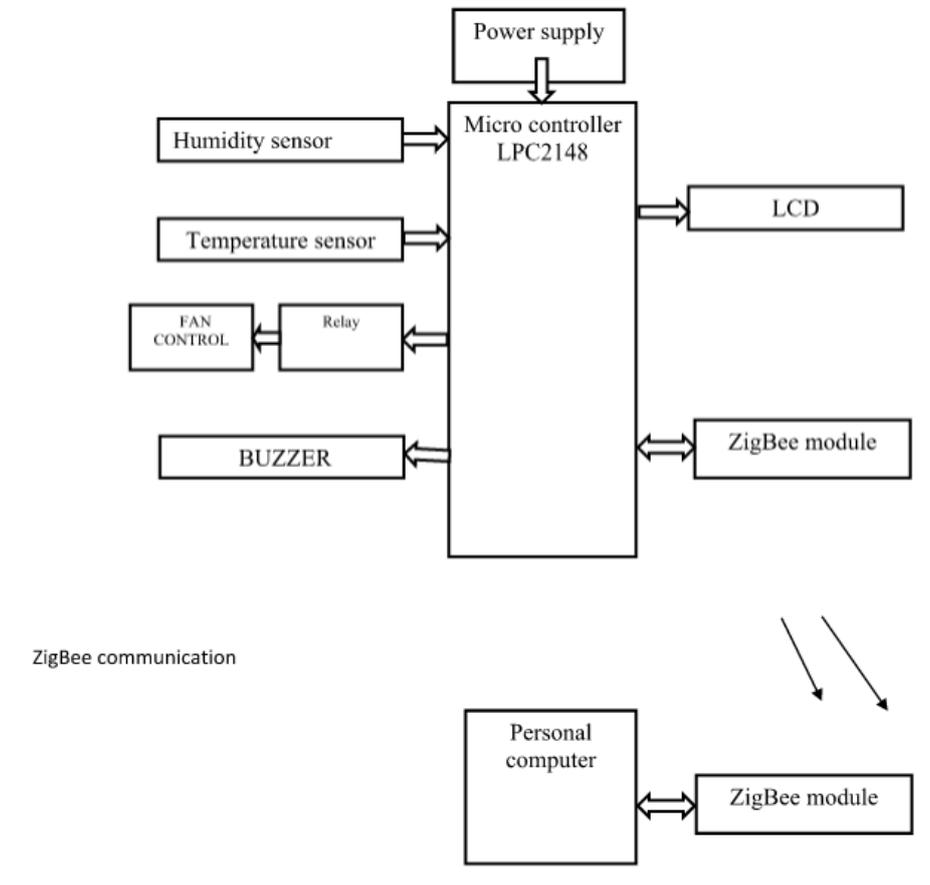
**Fig1: Transmitter and Receiver block diagram**
