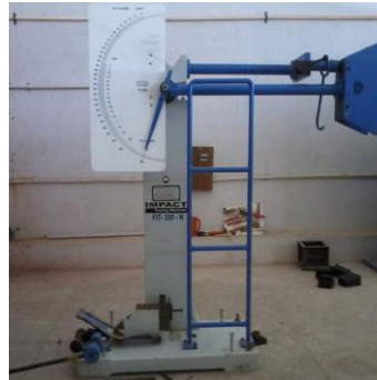
Figure 4.3: Impact testing machine ( Izod test )
