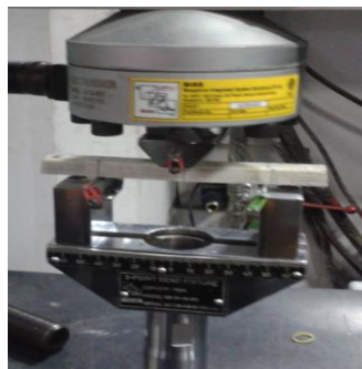
Figure 4.2: Flexural testing unit showing the positioning of sample
