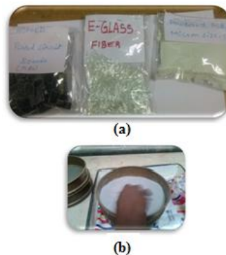
Fig.1 (a) Materials (b) PCB Powder Sieving Process
