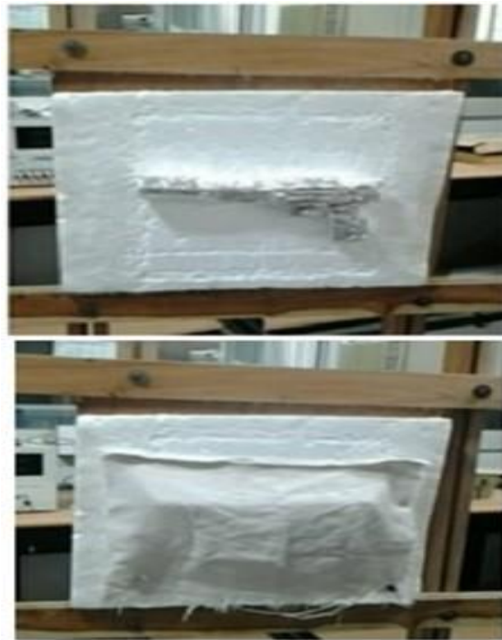
Fig.2. Target arrangement used for millimeter wave stand-off concealed weapon detection and identification (a) Toy gun, (b) concealed toy gun covered with cloth piece.
