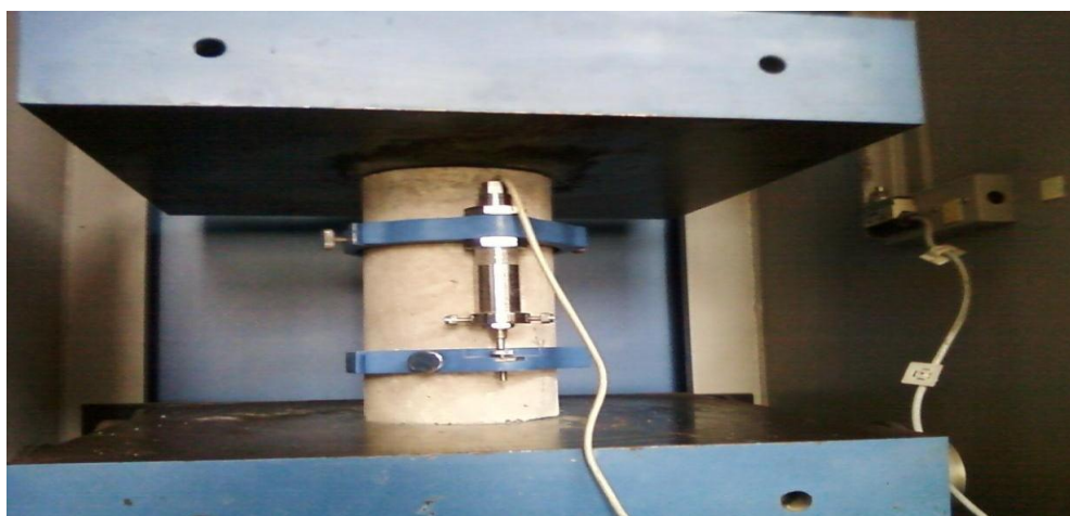
Fig.3.4 Set to draw stress strain curve by CTM using LVD
