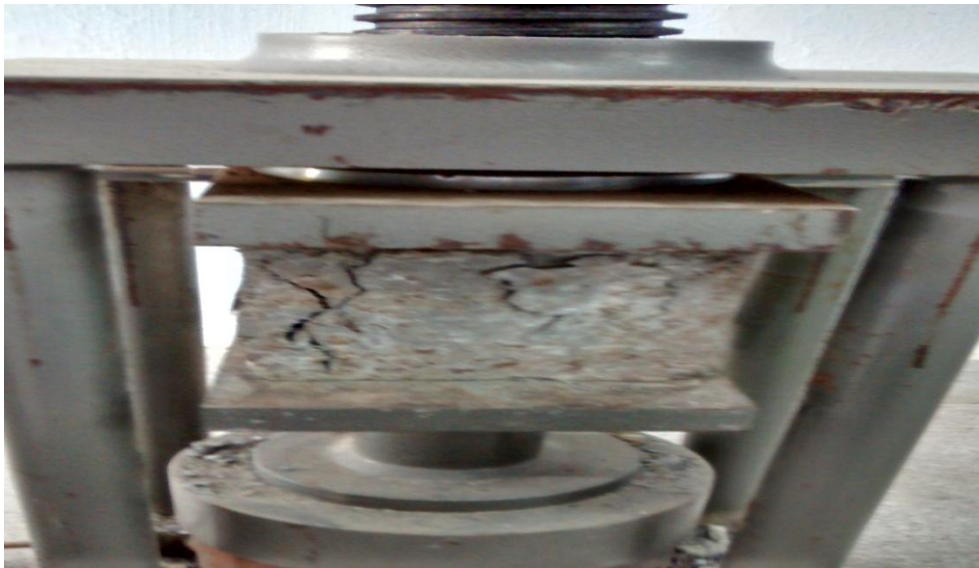
Fig3.5 Failure of sample under compression
