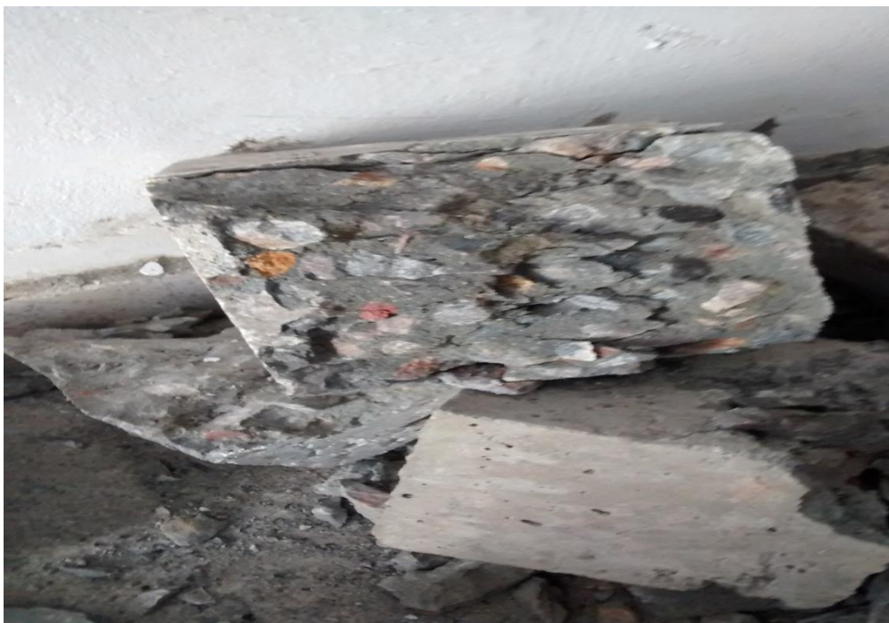
Fig 3.6 Failure pattern of samples under compression
