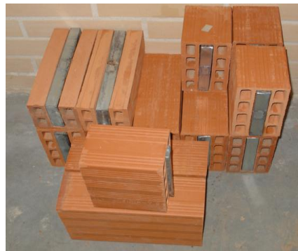
Fig6. Bricks with holes for PCM
