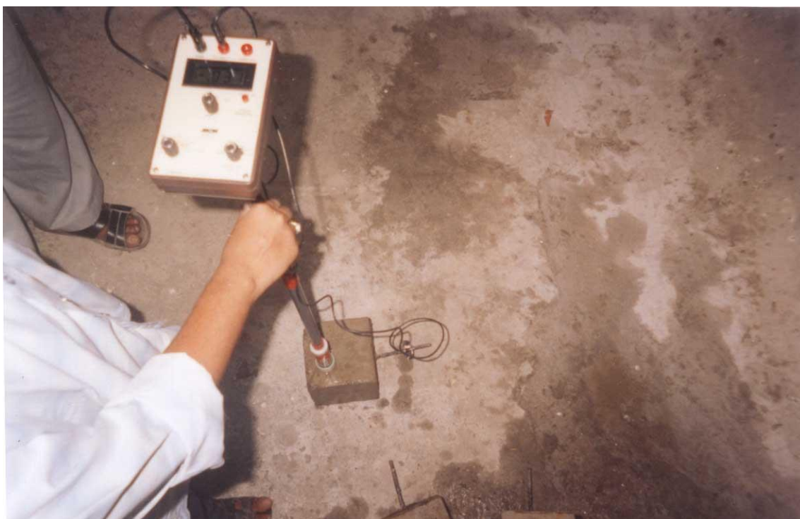
Figure 3 (b) Testing with Half-cell potentiometer
