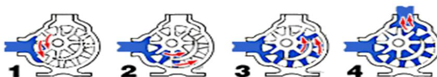
Fig.3.Working of Internal Gear Pump
