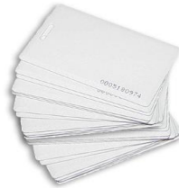
Fig. 3. RFID Tag (standard clamshell passive tag)
