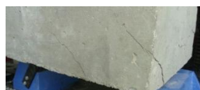
Plates-Crack Pattern in Bubble Deck Slab
