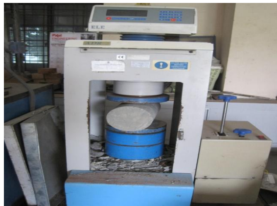
Figure 4: Split Tensile Test On cylinders
