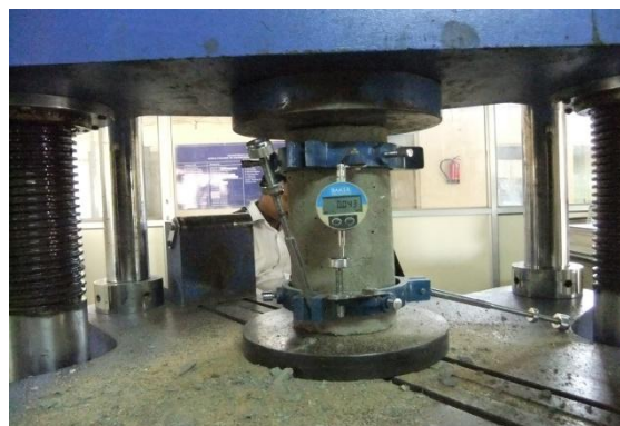
Figure 5: Axial Compressive test on Cylinders
