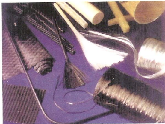
fig 3.2: Common glass and carbon fibers and FRPs used in structural engineering
