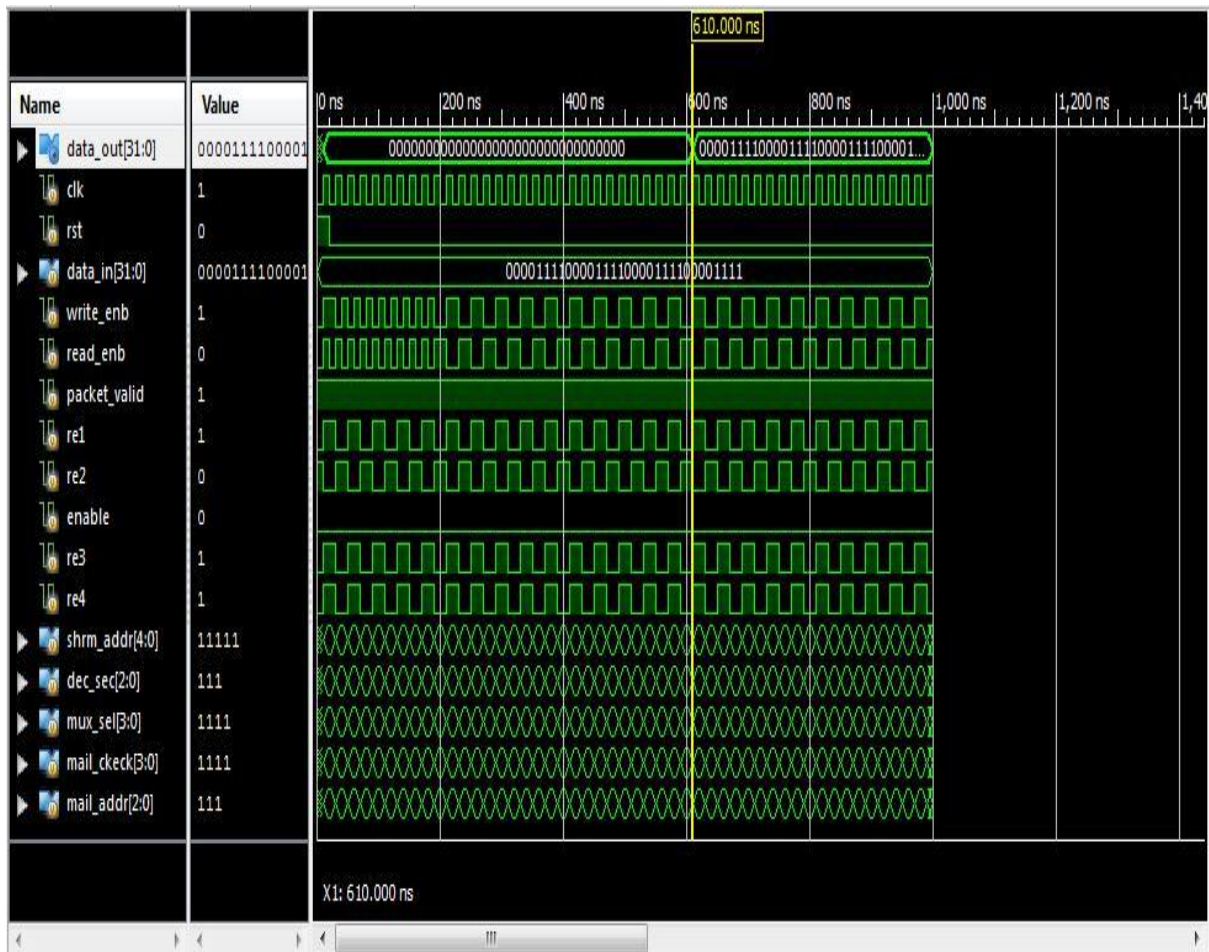
Fig. 9. Simulation results of shared-memory communication.
