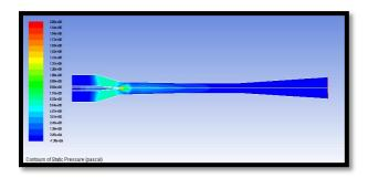
According to the above contour plot, the maximum static pressure inside of the steam ejector at nozzle because the applying the boundary conditions at inlet of the steam ejector nozzle and minimum static pressure at the steam outlet.
