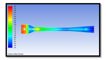
According to the above contour plot, the maximum Mach number at steam ejector nozzle and secondary fluid inlet because the applying the boundary conditions at inlet of the steam ejector nozzle and minimum static pressure at the steam outlet.
