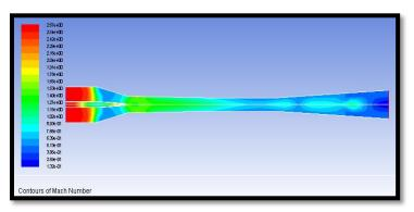
According to the above contour plot, the maximum Mach number at steam ejector nozzle and secondary fluid inlet because the applying the boundary conditions at inlet of the steam ejector nozzle and minimum static pressure at the steam outlet.
