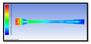
According to the above contour plot, the maximum Mach number at steam ejector nozzle and secondary fluid inlet because the applying the boundary conditions at inlet of the steam ejector nozzle and minimum static pressure at the steam outlet.
