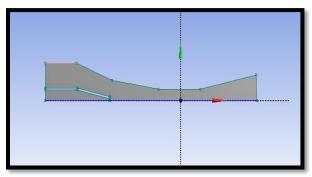
$\rightarrow \rightarrow$  Select mesh on work bench  $\rightarrow$  right click  $\rightarrow$  edit  $\rightarrow$  select mesh on left side part tree  $\rightarrow$  right click  $\rightarrow$  generate mesh  $\rightarrow$
