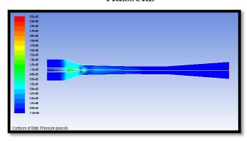
According to the above contour plot, the maximum static pressure inside of the steam ejector at nozzle because the applying the boundary conditions at inlet of the steam ejector nozzle and minimum static pressure at the steam outlet.
