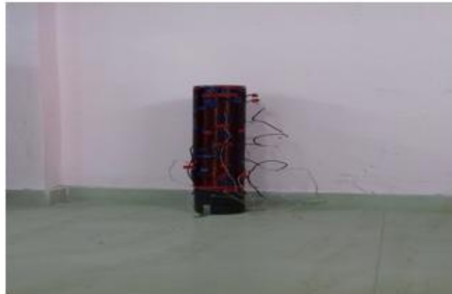
Figure1:- Electromagnetic model of HV winding of 60 MVA, 11 kV/230kV transformer.
