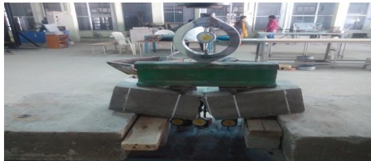
Figure 4:2 Flexural test on beams
