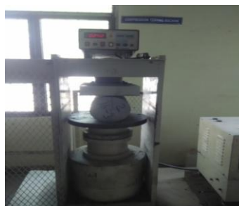
Figure 4:1 Split tensile test on cylinders
