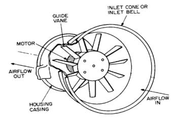
**2.2 Tube axial fan:** - Tube axial fan primarily propeller fan placed within the cylinder shell and its one diameter long generally. They generate higher pressure and better efficiencies as compared to axial fans. They are used in HVAC application. Its motor orientation will be either upstream or downstream of the blade. They are costly in construction and less noisy in operation as compared to axial flow fan. They are 65% energy efficient.
