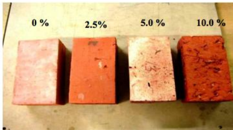
Figure 1. Surface texture of bricks for mixes with 0 %, 2.5 %, 5 % and 10 % CBs 2
