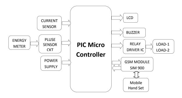
Fig. 1 Block Diagram of the Module
