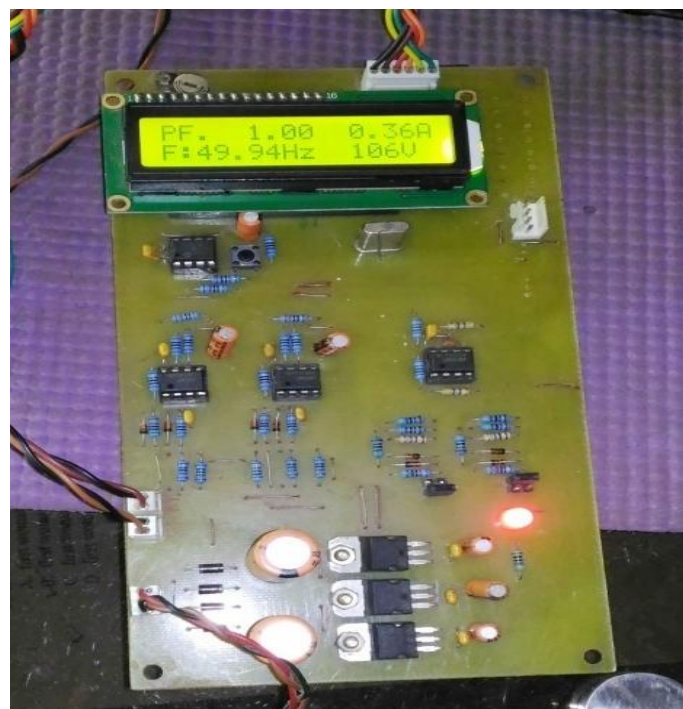
Fig.6 Hardware model with inductive load (corrected pf)
