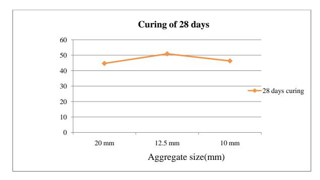
28 days Compressive Strength with various Sizes of Aggregates
