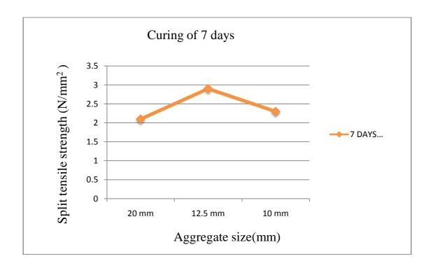
7 days Split Tensile Strength with various Sizes of Aggregate
