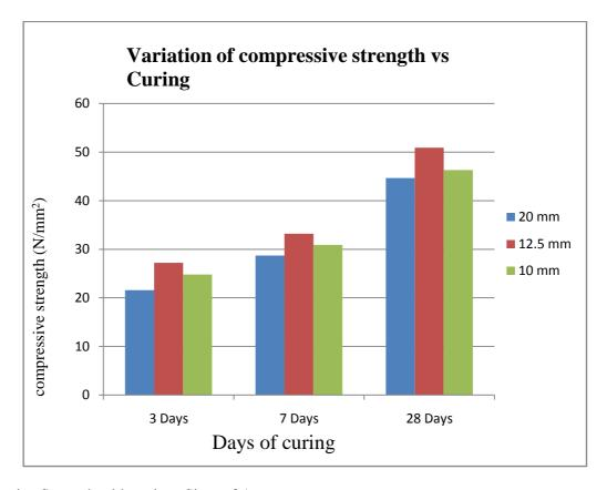
Compressive Strength with various Sizes of Aggregates
