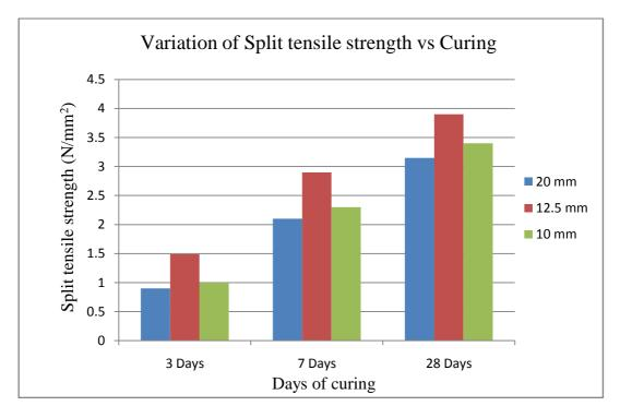
Split Tensile strength with various Sizes of Aggregate
