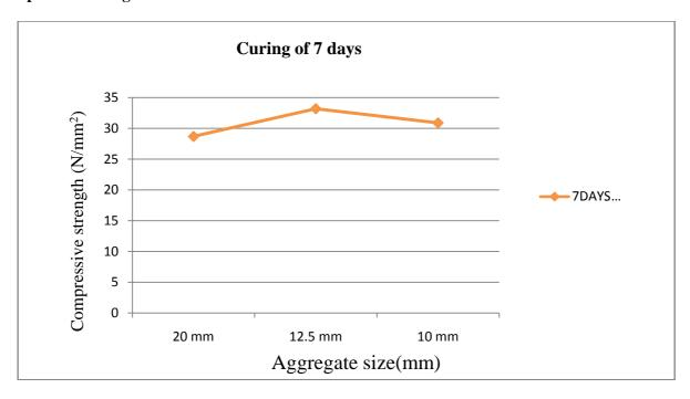
7 days Compressive Strength with various Sizes of Aggregates
