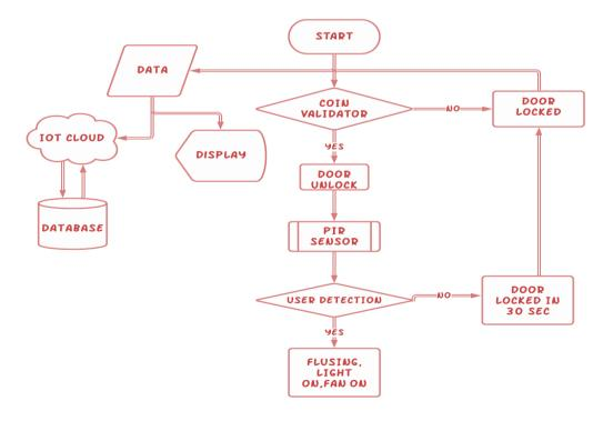
Fig.2.Flowchart explaining how IoT based E-toilet with Automatic Flushing and Sanitizing.
