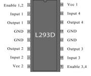
The motors are rotated on the basis of the inputs provided across the input pins as LOGIC 0 or LOGIC 1. In simple words we need to provide Logic 0 or 1 across the input pins for rotating the motor. Lets consider a Motor connected on left side output pins (pin 3,6). For rotating the motor in clockwise direction the input pins has to be provided with Logic 1 and Logic 0.
