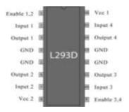
The motors are rotated on the basis of the inputs provided across the input pins as LOGIC 0 or LOGIC 1. In simple words we need to provide Logic 0 or 1 across the input pins for rotating the motor. Lets consider a Motor connected on left side output pins (pin 3,6). For rotating the motor in clockwise direction the input pins has to be provided with Logic 1 and Logic 0.
