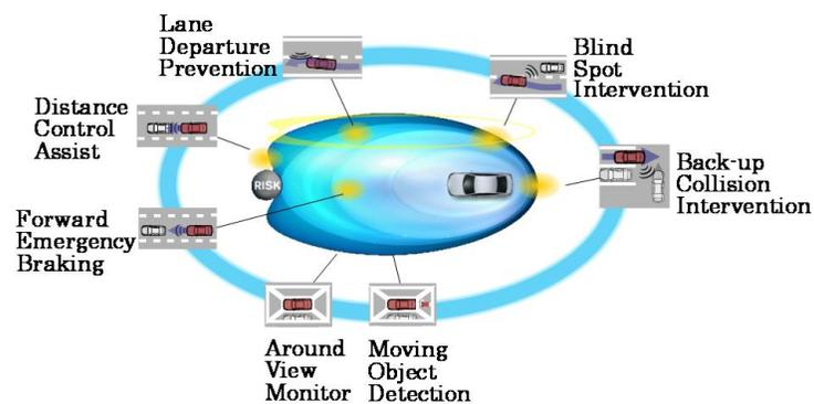
Fig. 8. All-around SAFETY SHIELD technologies
