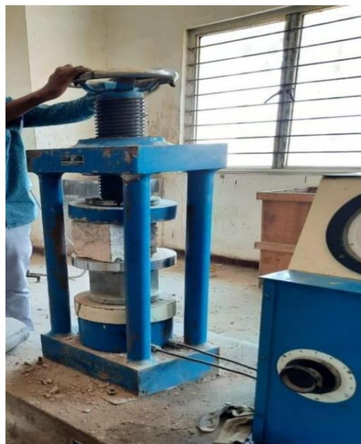
**Fig 4.1 - Test Setup for Compressive Strength**
