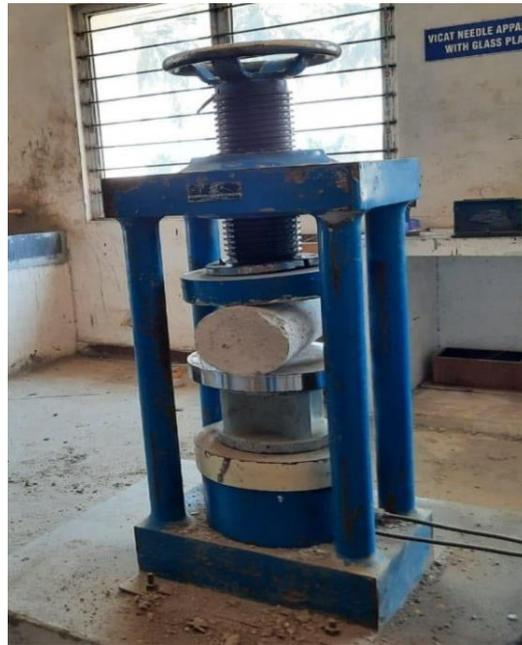
Fig 4.3 - Test Setup for Split Tensile Strength
