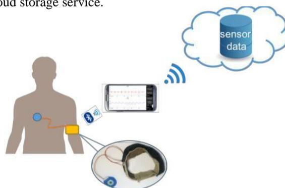
**Figure 3. A cloud-enabled wearable device for continually monitoring several physiological signals is depicted.**
