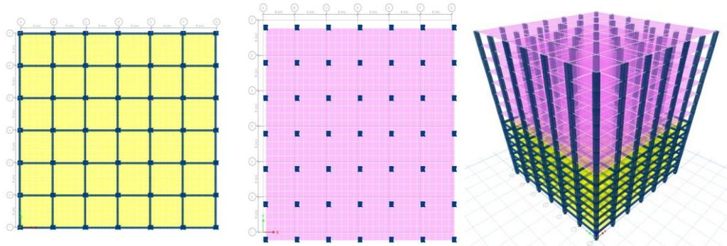
Figure 8: a. Plan view from Ground storey to 7<sup>th</sup> storey, b. Plan view from 8<sup>th</sup> storey to 15<sup>th</sup> storey and c. Elevation view of model CS+FS
