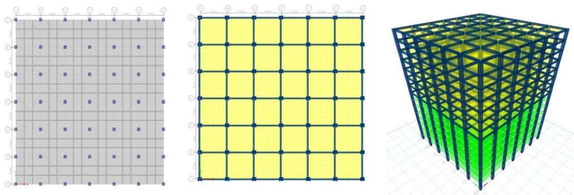
Figure 6: a. Plan view from Ground storey to 7<sup>th</sup> storey, b. Plan view from 8<sup>th</sup> storey to 15<sup>th</sup> storey and c. Elevation view of model GS+CS
