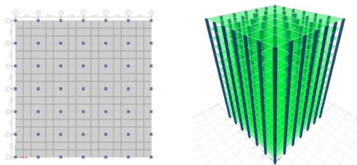
Figure 10: a. Plan view and b. Elevation view of model GS
