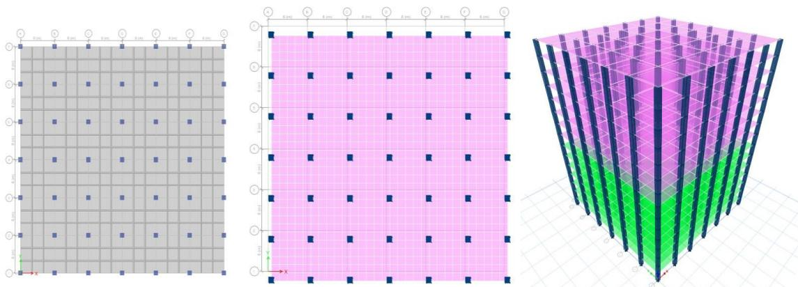
Figure 9: a. Plan view from Ground storey to 7<sup>th</sup> storey, b. Plan view from 8<sup>th</sup> storey to 15<sup>th</sup> storey and c. Elevation view of model GS+FS
