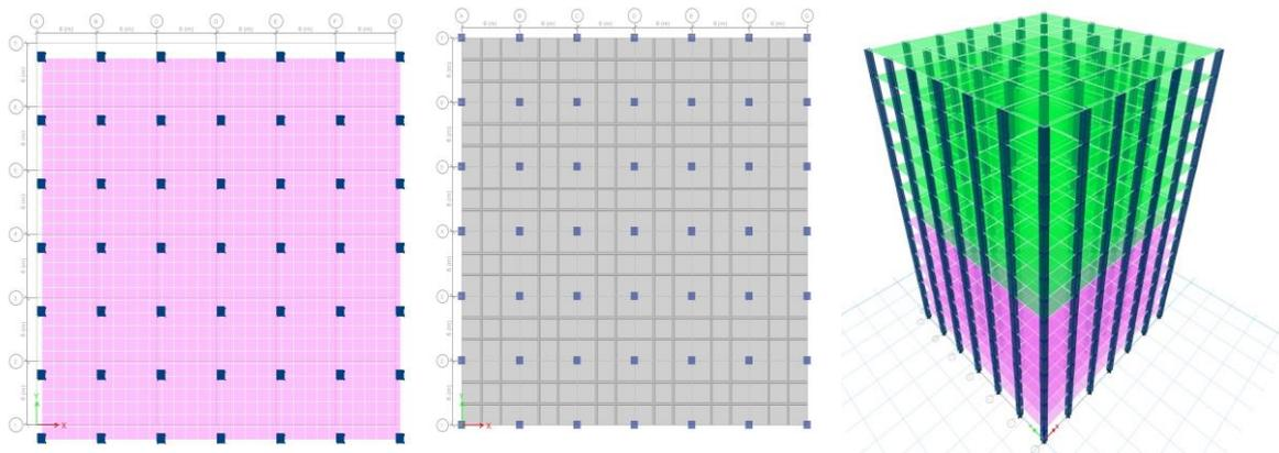
Figure 12: a. Plan view from Ground storey to 7<sup>th</sup> storey, b. Plan view from 8<sup>th</sup> storey to 15<sup>th</sup> storey and c. Elevation view of model FS+GS
