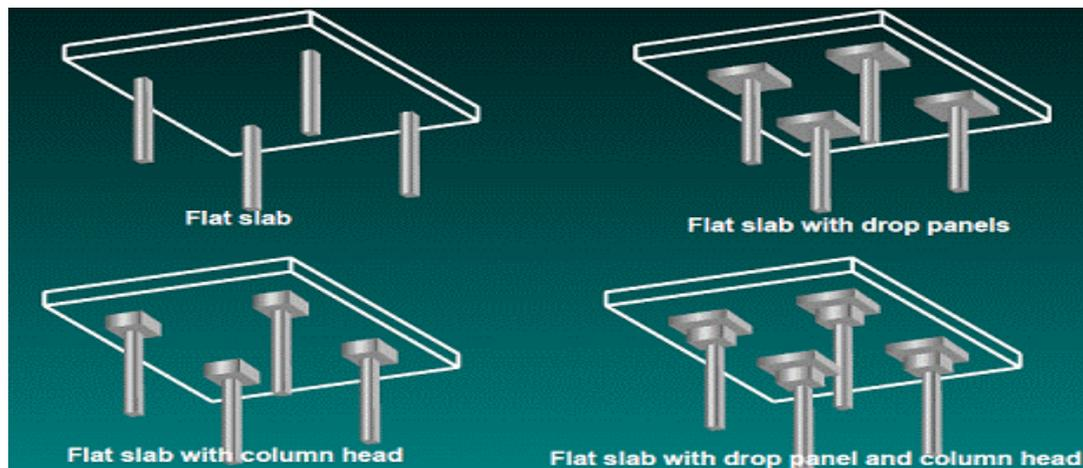
Figure 2: Types of Flat Slab [9]
