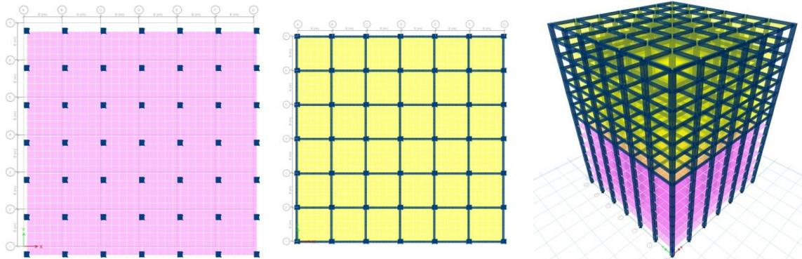
Figure 5: a. Plan view from Ground storey to 7<sup>th</sup> storey, b. Plan view from 8<sup>th</sup> storey to 15<sup>th</sup> storey and c. Elevation view of model FS+CS
