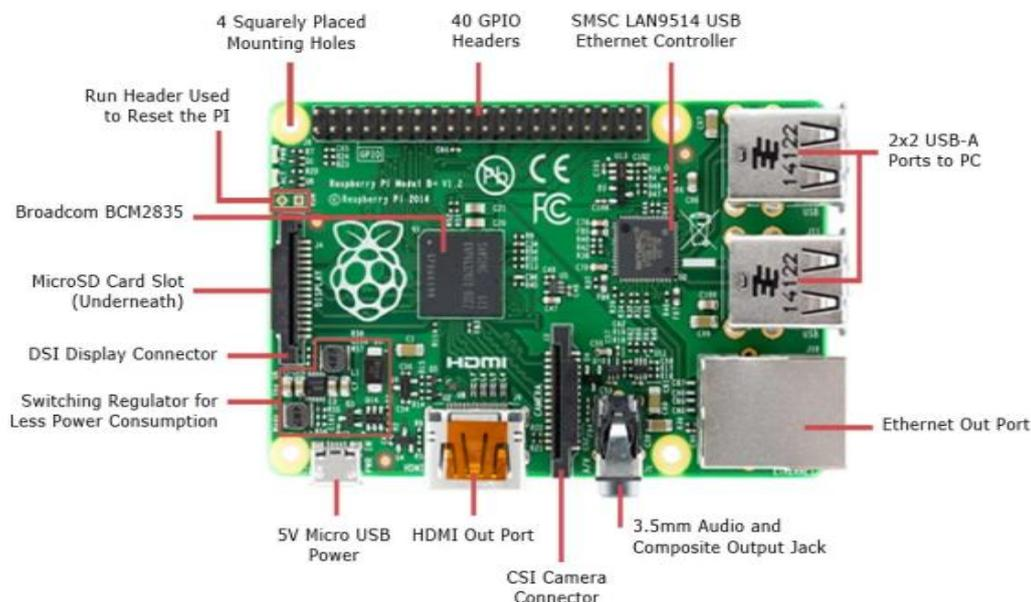
Fig .2. Raspberry Pi board
