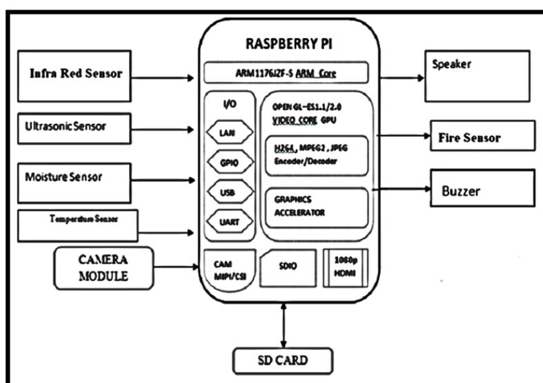
Fig.1. Block diagram of blind stick
