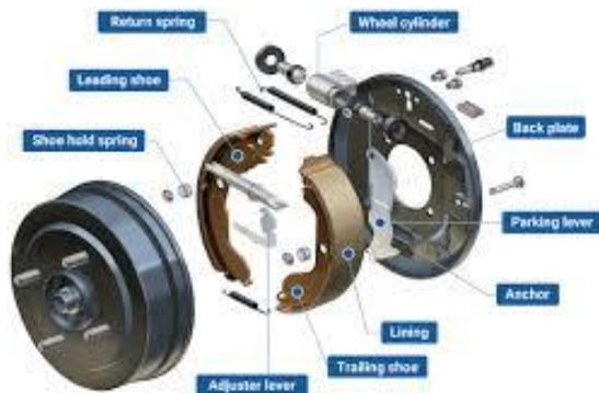
Fig.5. Drum Brake
