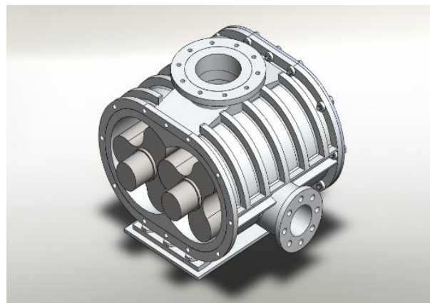
Figure 5: Roots blower (The final product)
