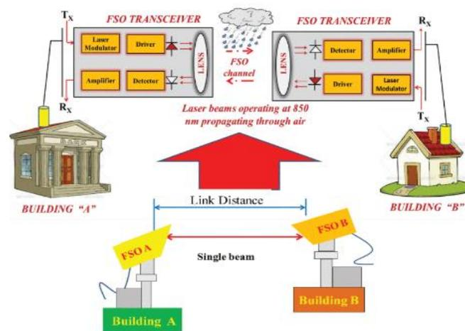
Fig. 2. Components of FSO System
